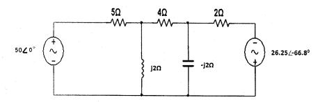
b) Find the value of load impedance 'Z' for which power transfer is (06) maximum in following circuit for w =400 rad/s & also value of max power transferred to the load.
