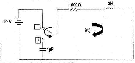
b) For series RLC circuit (as shown in figure below), the capacitor is (06) initially charged to Ivolt, find the current i(t), when switch k is closed at t= 0 Using Laplace transform.
